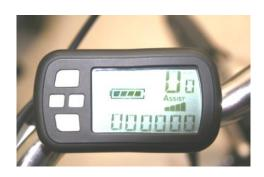
There are less bars visible the less the Battery is charged. When the last remaining bar is flashing, this means that the Battery will be completely discharged soon.
