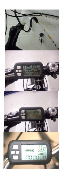
The actual speed is shown in the upper right edge as Km/h.
