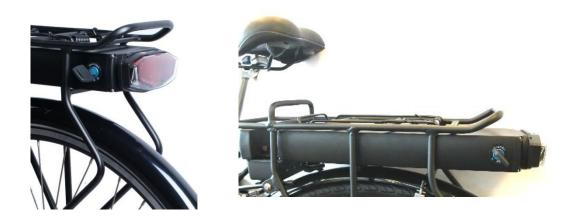
Turn the key (ON/OFF) to open position and take the battery out of the rear rack.
